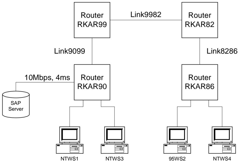
Figure 5-1: Topology setup in ns
