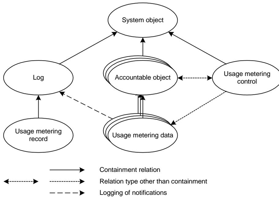
Figure 6-2: Example of structural relationship of managed objects
